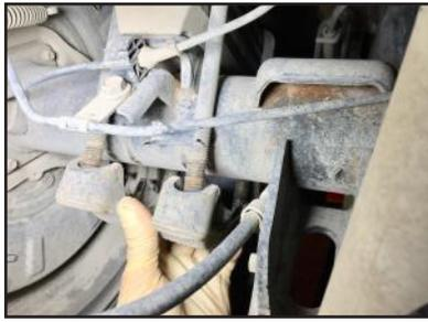
**STEP 6:** Lift vehicle by frame or leaf spring. Remove factory rear block.
