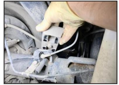
**STEP 7:** Install desired amount of lift. Make sure alignment pins line up with spring and axle. Make sure **FRONT** marking on block is facing **FRONT** of vehicle. Utilize lower portion of block to get 1.0" rear lift as shown here.
