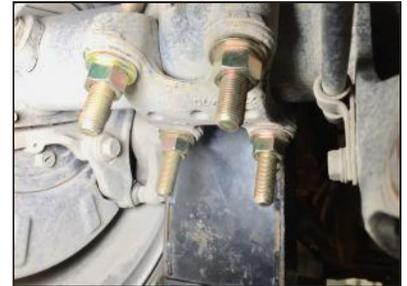
**STEP 11:** Install shock bolt and nut. Torque to manufacturer's specifications.
