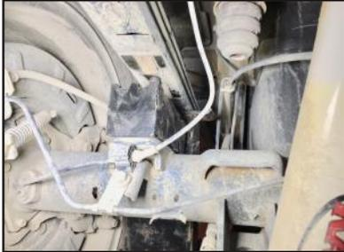
**STEP 8:** Utilize two lower blocks together to get 1.5" rear lift as shown here.
